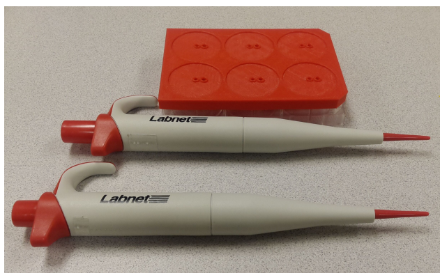
Figure 1: 3-D printed micropipette guide for six well plate (at top) and two fixed volume micropipettes (bottom) assist BLV users in dispensing liquids with less tactile probing
