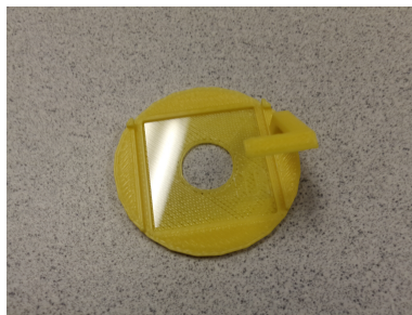
Figure 2: 3-D printed glass microscope coverslip holder with indentation to hold the coverslip in place. The diameter of the holder is equal to the diameter of the wells
